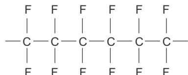
**PFA :** Perfluoroalkoxy, or PFA, is probably the most commonly applied valve liner or molded lined products . PFA is very similar to modified PTFE in that is has an additive of PPVE except the amount is increased from 1% to 4%. Chemical compatibility and temperature capabilities are unchanged but mechanical properties are changed. The most significant change results in this material now being able to be melt-processed.
