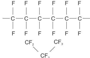
**FEP :** Perfluoroethylenepropylene, or FEP, is another commonly applied valve liner. FEP is made from tetrafluoroethylene and approximately 15 - 20 % hexafluoropropylene. Its chemical resistance is nearly the same as PTFE, Modified PTFE and PFA; however its thermal resistance is less than PTFE or PFA.
